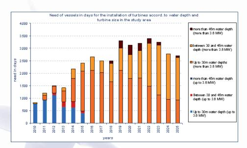
offshore wind turbines is a real challenge to logistics as high requirements have to be met. Particularly, a high need of special vessels for the transport, installation and maintenance of offshore wind turbines becomes evident.
